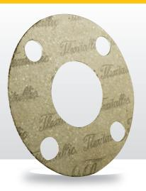
Thermiculite<sup>®</sup> 815 is a high temperature, chemically resistant sheet sealing material comprising exfoliated vermiculite reinforced with a tanged stainless steel core.
